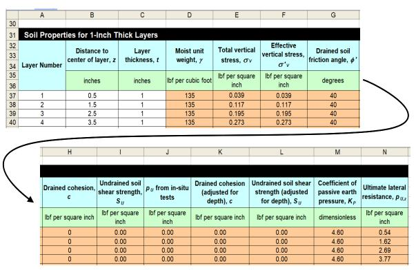
Figure 6. Soil properties table for 1-inch thick soil layers.
