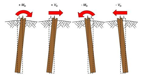
Figure 11. Sign convention for groundline bending moment  $M_G$  and shear force  $V_G$ . When  $M_G$  and  $V_G$  are induced by an ASD load combination they are written as  $M_{ASD}$  and  $V_{ASD}$ , respectively. When  $M_G$  and  $V_G$  are induced by an LRFD load combination they are written as  $M_{LRFD}$  and  $V_{LRFD}$ , respectively.
