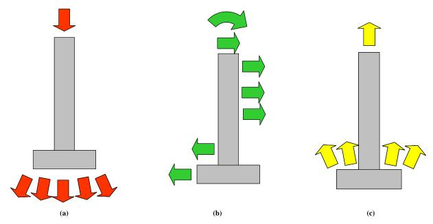
$Figure \ 1.\ (a)\ Bearing\ load,\ (b)\ lateral\ load,\ and\ (c)\ uplift\ load\ on\ a\ shallow\ pier/post\ foundation.$
