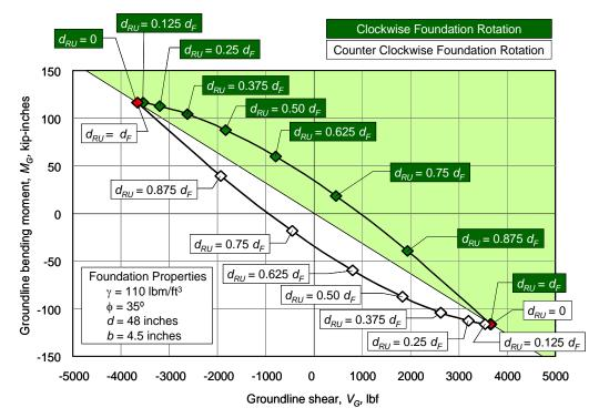
Figure 14.  $V_U - M_U$  envelope from ASAE EP486.3 showing relationship between  $M_U$ ,  $V_U$  and the location of the ultimate pivot point  $d_{RU}$ .
