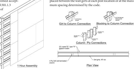
Figure 1. Post-frame fire-rated wall assembly details (from UL design V304)
