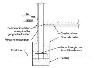
Figure 2. A constrained shallow-post foundation with a concrete collar and a concrete floor
