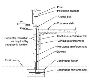
Figure 3. A continuous concrete wall foundation with a concrete floor. Posts are attached to the foundation with post base brackets.
