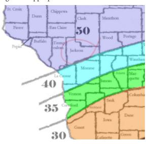
Figure 1 – A portion of Wisconsin's Ground Snow Load Contours from ASCE 7 shows most of Jackson County is clearly in a 50 psf region (not the 35 psf used)
