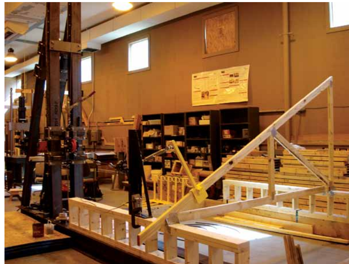
Figure 3 Horizontal application of load test (HALT), with test truss mounted using eave bracket
