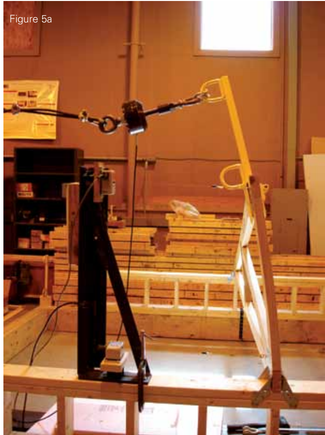
Figure 5 Sequential testing of loading showing anchor attachment to truss (eave bracket)
