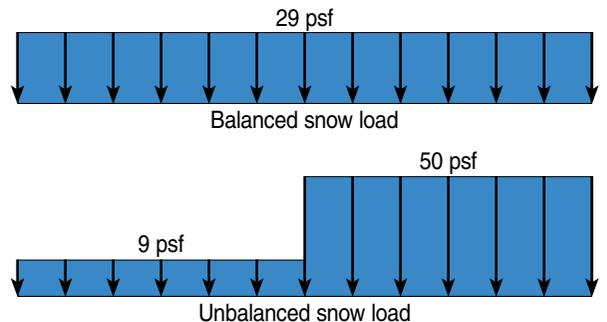
conditions of the roof,  $C_s$  is determined using the slope of the roof in degrees (or pitch) and either the dashed line for unobstructed slippery surfaces or the solid line for all other surfaces. It should be noted that Section 7.4 states that the sloped roof snow load is assumed to act on the horizontal projection of the roof
