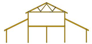
Figure 1-53. Primary frame of a building with clerestory.
