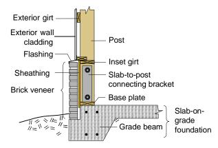
Figure 1-21. Slab-on-grade foundation.
