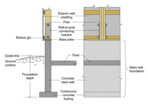
Figure 1-25. Stem wall foundation.
