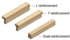
Figure 1-20. Types of individual member reinforcement.
