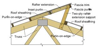
Figure 1-15. Overshot ridge with rafter extension supported by a two-ply rafter extension support. One ply is located between the rafter extension and truss top chord; the second ply extends along the sides of the rafter extension and truss chord.
