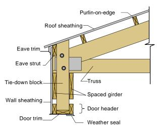
Figure 1-12. Cross-sectional view through an overhead door in the sidewall of a building without an eave overhang.
