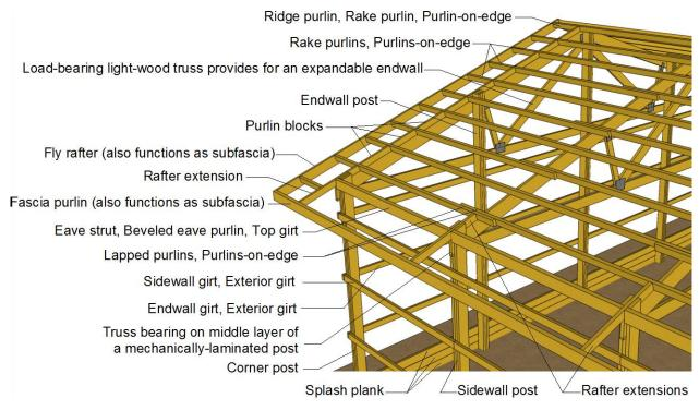
Figure 1-10. Typical corner framing.
