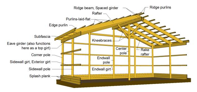
Figure 1-11. Section of a post-frame building featuring girder-supported rafters. Although posts of any type can be used to support girders, this image shows round poles being used as structural wood columns.
