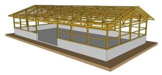
Figure 1-2. Post-frame building mounted on a concrete stem wall.
