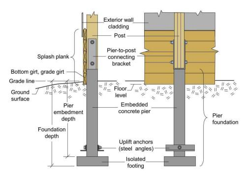
Figure 1-24. Pier foundation featuring steel angles for uplift anchorage.
