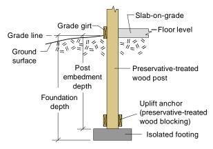
Figure 1-22. Post foundation featuring a preservativetreated wood blocks for uplift anchorage.
