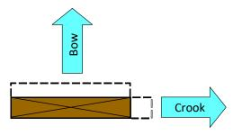
Figure 1-26. Lumber warping terminology: bow versus crook as viewed from end of wood member.
