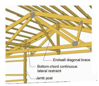
Figure 1-19. Endwall diagonal brace used to transfer endwall forces into roof diaphragm and to keep bottom chord continuous lateral restraint from shifting.
