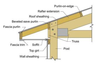
Figure 1-13. Cross-sectional view through an eave overhang that is supported by a rafter extension that runs continuously from the edge purlin/sub-fascia to the first purlin above the post. The rafter extension is fastened to the post, purlin, and top of the truss.
