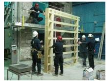
An hourly rated wall—rated as high as 3 hours—is often required to separate building areas or occupancy types to meet the *IBC* requirement for life safety. For architects, builders, and engineers, that traditionally has meant using a rated 8-inch or 10-inch concrete block wall on a concrete foundation, but with this recent test exceeding hour-rating expectations, that may no longer be the case.
